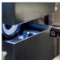
QCam 360 The camera system checks the cable ends; reject parts are sorted out immediately and automatically reproduced.
