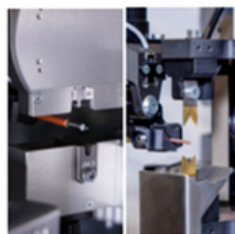
Cutting and sawing The blade system features block, single and multi-blade heads. The sawing unit cuts cables quickly and at a perfect right angle. The inner conductors remain absolutely straight.
